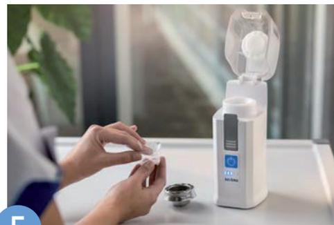
**5** Check the grinding head for visual contaminations. Gently remove the SeveroRondel, check for damages and tap off any remaining medication before disposal.
