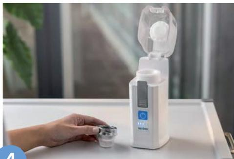
**4** After grinding, open the lid and take out the SeveroCup together with the grinding head. Check the cup for visual contaminations. Remove the grinding head while keeping the SeveroRondel in the cup.
